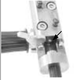
On completion of flanging
