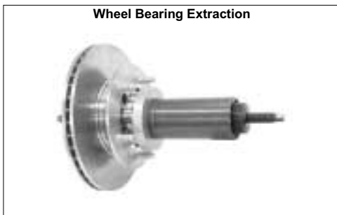
Wheel Bearing Extraction
